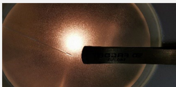
Figure 4. Open the orifice of the emitter using a tweezers under microscope
